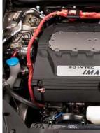
High-Voltage Cable Connection to Motor
