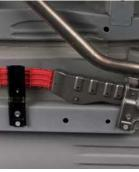
Electrical shield bolted to undercarriage
