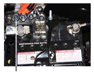
DC to DC Converter Cable Connection
