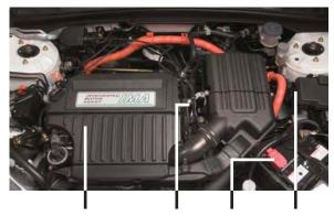
Engine Motor 12-Volt Underhood Battery Fuse Box
